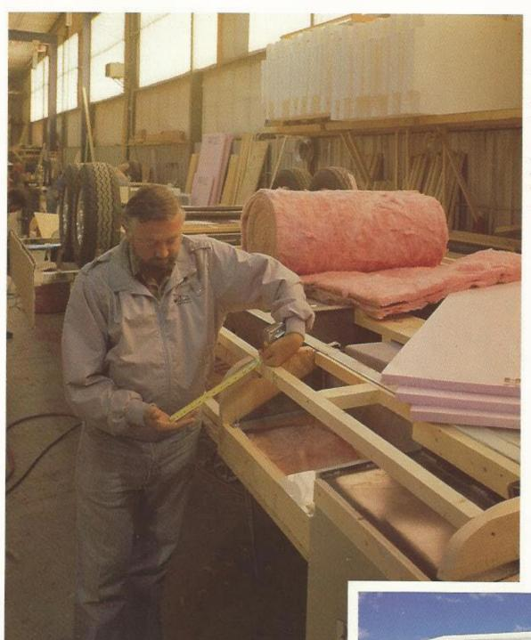
Teton builds one of the thickest, most durable floor/frame systems in the industry. An 8" I-beam substructure, 2"x4" floor joists, plus 3/4" tongue and groove plywood flooring provide over 12" of thickness. Not only is this the strongest floor/frame system available, it is the best insulated.
