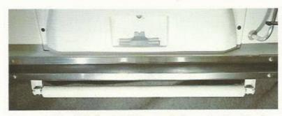
This 62" wide skid roller is a Teton exclusive — designed and built right at the factory. This heavy duty roller will end any worries you might have about damaging the underbelly of your trailer. Built Wyoming tough.
