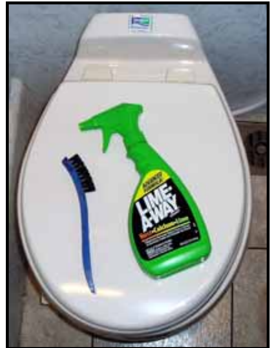
A stiff bristle brush or bottle brush, and mineral dissolving product are necessary to clean the ball valve and seals.
