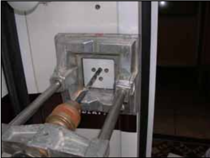
Drilling outside-in: I used a special drilling jig (from Sears) to make sure all holes were perpendicular
