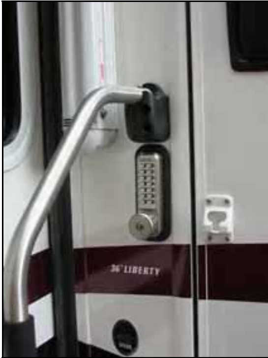
Exterior: Our lock has a key over-ride. When our fifth wheel goes in for service, we hand the mechanic the key---no need to reset combo after servicing rig.
