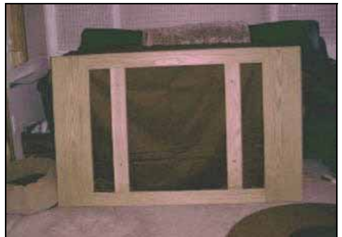
This is the oak frame that covers the original TV and component cabinets. Center uprights are placed so that the new TV can be mounted on to the front of the frame.
