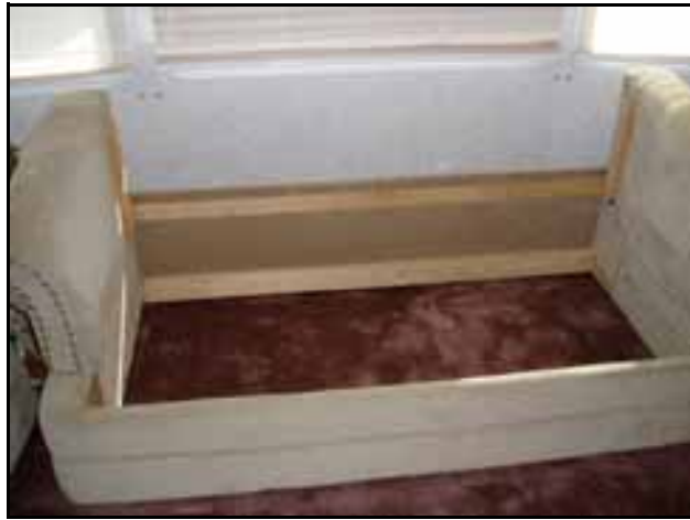
Figure 2— This is the couch with the bed mechanism and the backrest removed. It is now ready to receive the storage box.
