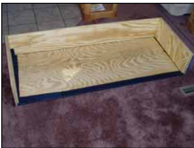
Figure 6 — Both side sections are put in place and attached to the rear brace board.
