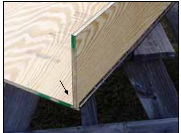
Figure 4 — Notice that the back extends the bench seat by 1/2 inch on each end and that the back sits on top of the bench seat when upside down.
