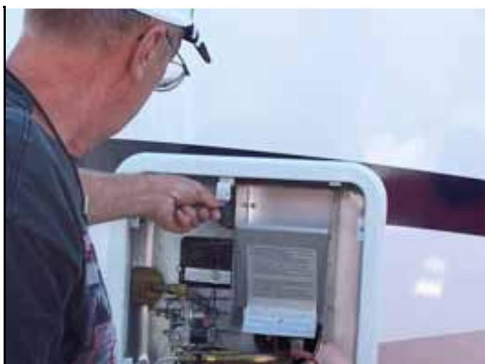
John Geldorf #683 releases a pressure valve during a demonstration on how to maintain and clean your hot water heater.
